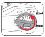
CAUTION: IF YOU TRY TO ROTATE THE CHAIN TENSIONING ADJUSTMENT DIAL WHILST THE CHAIN COVER LOCK IS TIGHT, IT WILL RESULT IN THE CHAIN NOT LOOSENING AND POSSIBLE DAMAGE TO THE MECHANISM.
