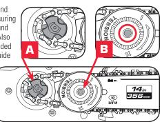
5. Attach the side cover and secure it with the side cover lock. Do not fully tighten the guide bar lock knob until after adjusting the chain tension.
