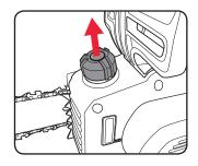
2. Fill the tank with chain bar oil. The capacity of the chain oil tank is 225ml. Do not over fill.
